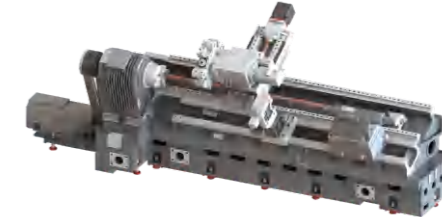
BG1000-10DW | Driven Tool Turret Tailstock
